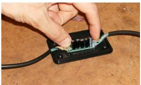
Photo 4: Press the board of the Cable onto the spots of glue
