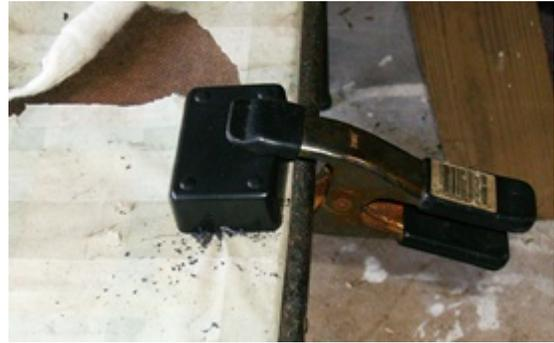
*Photo 1: Clamping down and drilling the hole.*
